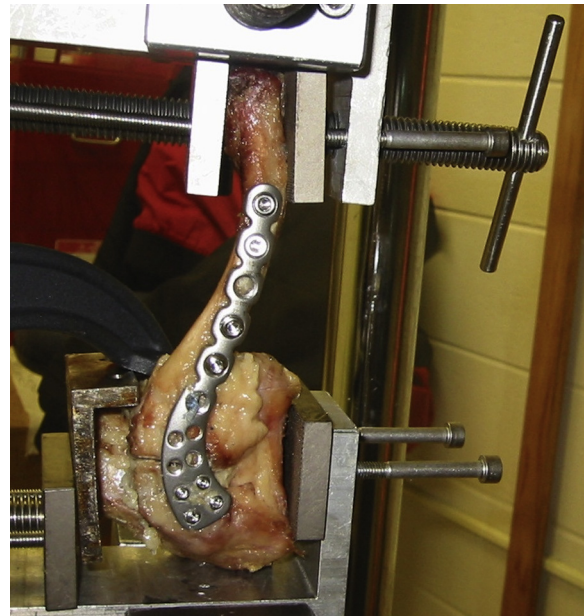
Figure 1 Jig for cyclic test and load to failure in tension.
